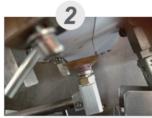
2: Box sucking and shaping
