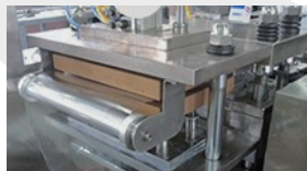
B. PVC/PET Heating and Forming
