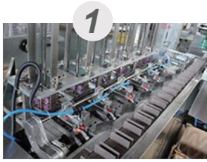
1: Product sucking and feeding into the conveyor
