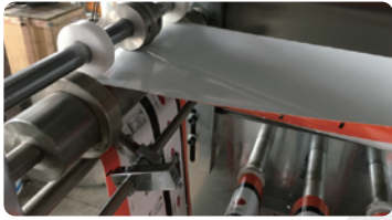
1 Packing Material Unwinding and Folding
