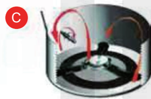
C. The process for the granules to be round and enlarged in the chamber (Floating)
