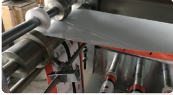
1 Packing Material Unwinding and Folding
